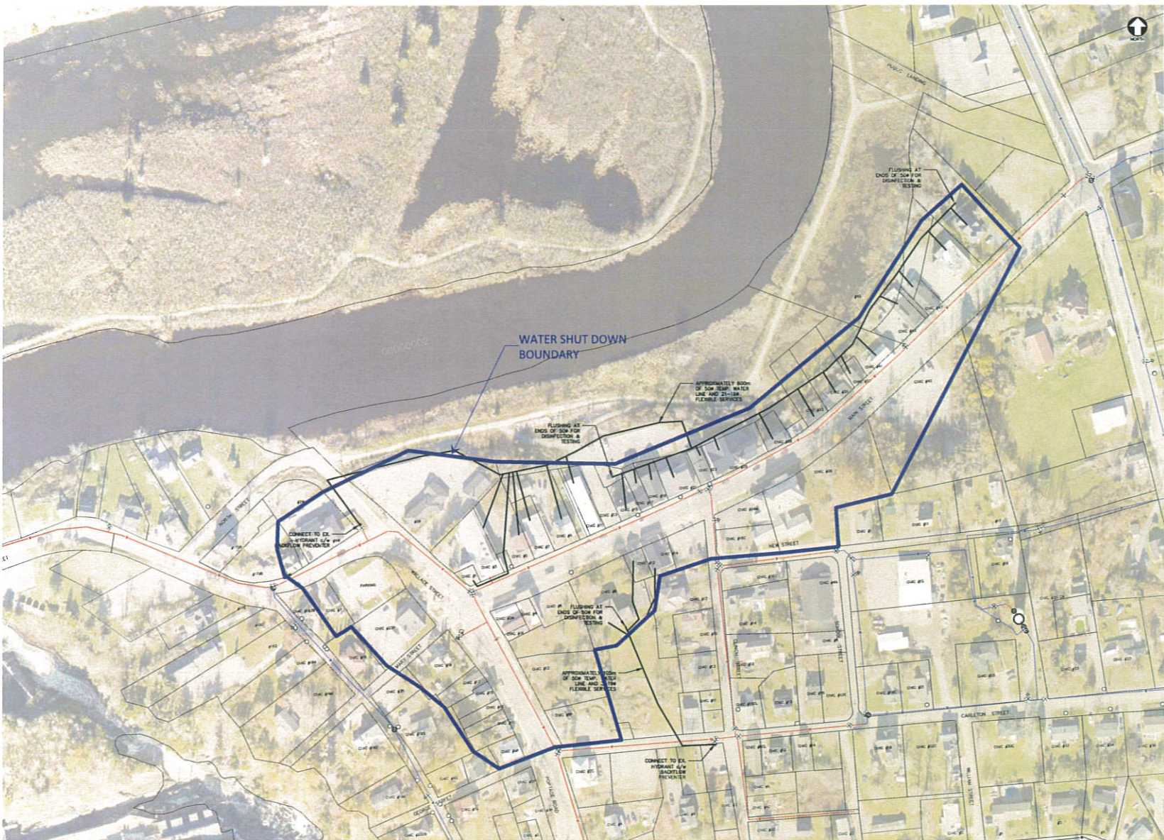
SITE PLAN—MAIN STREET — TEMPORARY WATER 0 20 40 60 80 100m 1:1000
